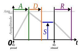
It is recommended that envelopes be *normalized*, with max *y* values reaching 1, and then scaled according to needs. Using the numerical coordinates in the EnvLib function, the range of *y* values can be extended: in the case of the <u>glissando</u> feature, for example, max *y* values need to exceed 1. The max *x* value will be automatically extended or compressed to correspond to the duration of the sound if the envelope reflects the evolution in time of a parameter.
